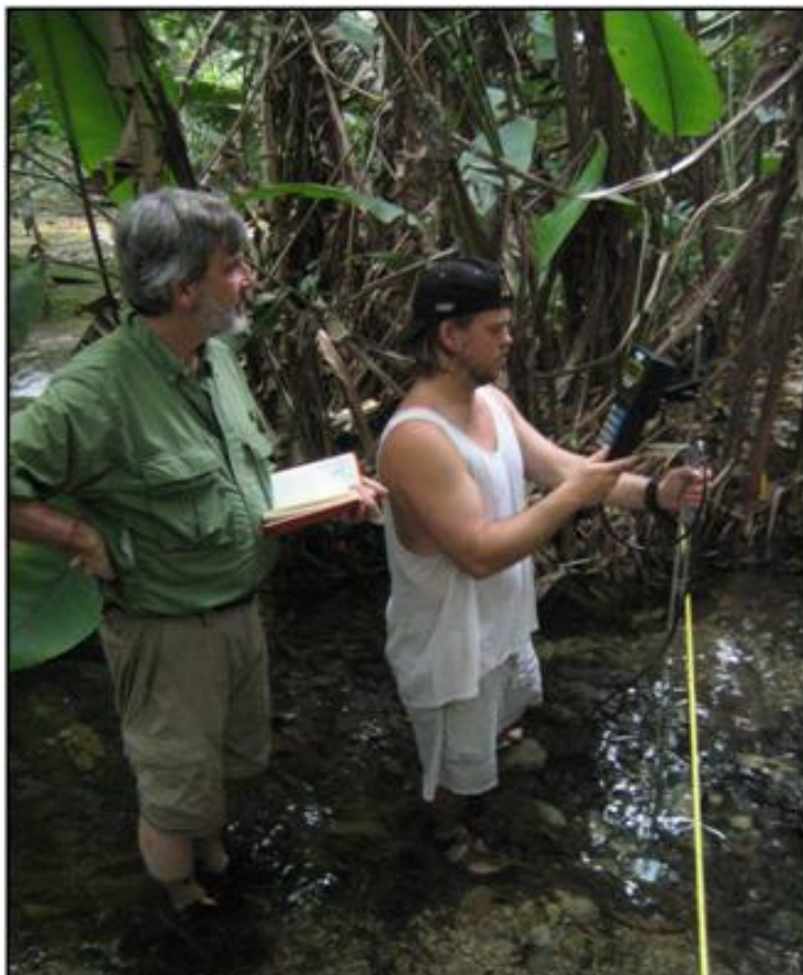
Figure 1.13 – – Dr. Christopher Duffy and Kirk French gauge the Picota Stream with the SonTek Flow Tracker.
